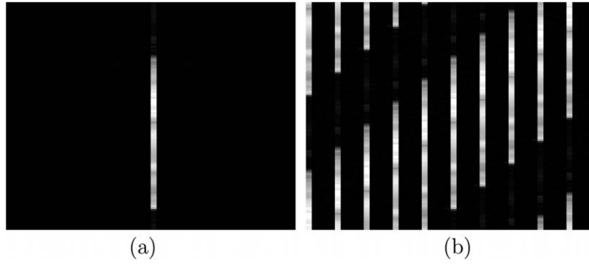
Fig. 4. Typical y - f maps obtained from k -space data acquired with an acceleration factor of 5 using: (a) Densely sampled low k -space (training data). (b) Undersampled full k -space (actual data).
